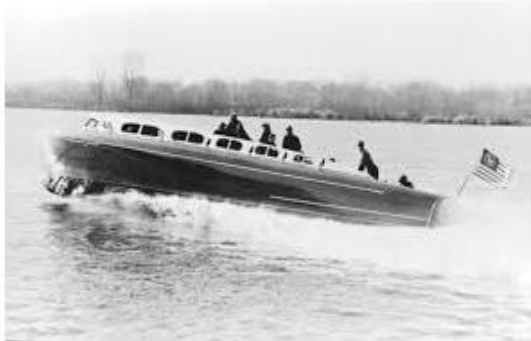
Whittell's 1940 mahogany 55' Thunderbird Yacht built by Hacker-Craft in Bay City, MI; twin 550hp engines raced around Lake Tahoe at 70mph with the likes of Sammy Davis, Jr., Tony Bennett, and Frank Sinatra
